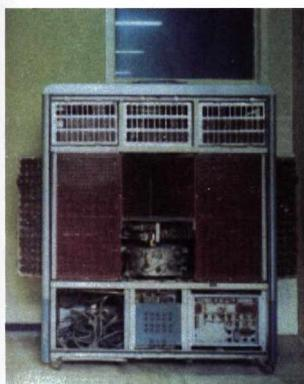
Fig. 1 – CRC 102-A. (1954) Drum memory is placed in central position. (Preserved at the Polytechnic of Milan)
