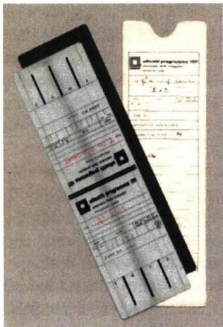
Fig. 13 – Floppy card for P 101; the black reverse is the magnetic-sensitive side. (7x25 cm)
