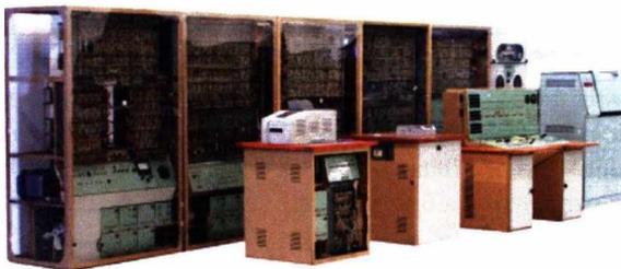
The Minsk computer family manufactured in Minsk for 10 years is practically speaking the descendant of the vacuum tube M3 computers developed in Moscow. The first member of the family, the Minsk 2, was the first semiconductor computer of the Soviet Union, the Minsk 22 is the already corrected and updated version of this. The one on exhibit was bought in 1968 by the National Committee for
